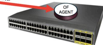
...a Layer 2 communications protocol that gives access to the forwarding plane of a network device,
